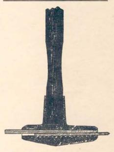
This advertisement shows the unique type of mill pick D.J. Hanford ordered. The drawing shows how the replacable tips were held in place.
